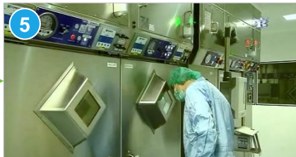
5 Radioactive liquid is dispensed by automatic dispenser
