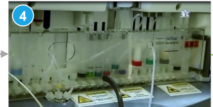
4 The cartridge and fluorine are put inside the synthesis module
